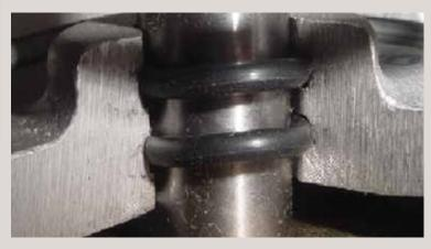
A worn center seal is one of the leading causes of spring brake leakage.
