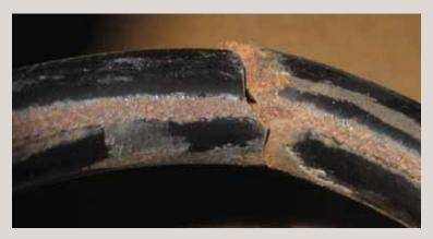
A broken power spring is the leading cause of spring brake failure.
